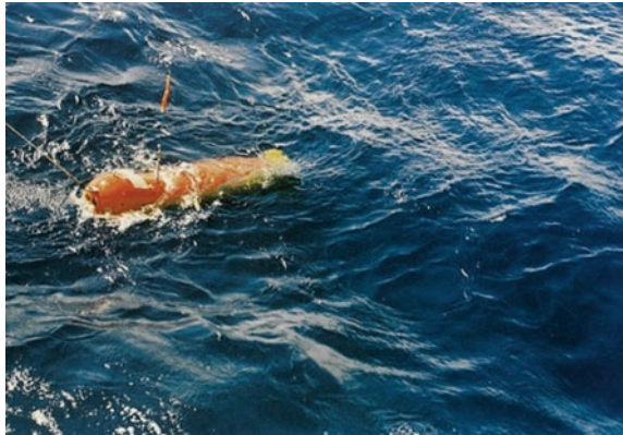
Fig. 6.6 CR-01 underwater vehicle [6]
