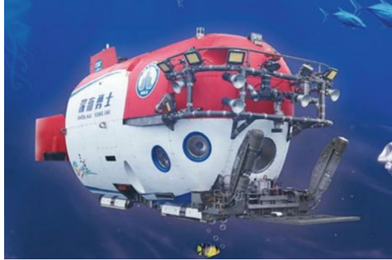
Fig. 6.9 “Shenhaiyongshi” deep-sea manned submersible [9]
