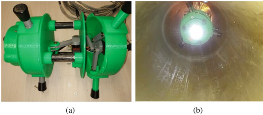
Fig. 9.5 Details of PEIS at DIMEG, University of Calabria: a view of the back module assembly; b view with the onboard lighting in dark conditions
