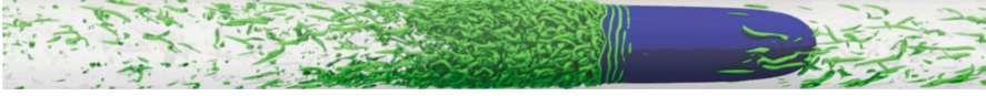
Fig. 2. Coherent turbulent structure visualization using iso surfaces (green) of the \lambda_2 criterion of the instantaneous velocity field. The bubble is represented by an iso surface (blue) at f = 0.5 .
