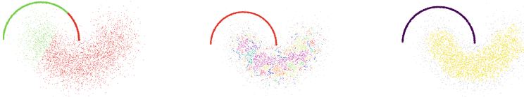
Fig. 3. Adapted Two Moons dataset with varying densities. [left] k-means partition. [center] DBSCAN partition. [right] mkNN-based partition
