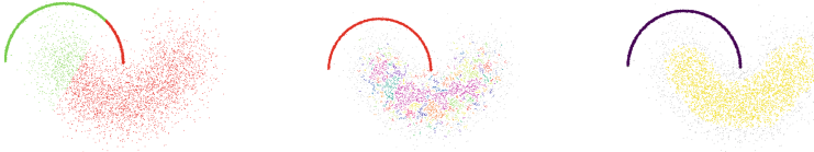
Fig. 3. Adapted Two Moons dataset with varying densities. [left] k-means partition. [center] DBSCAN partition. [right] mkNN-based partition
