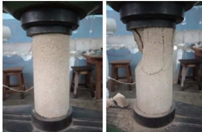
Fig. 4. Sand based backfill during UCS test.
