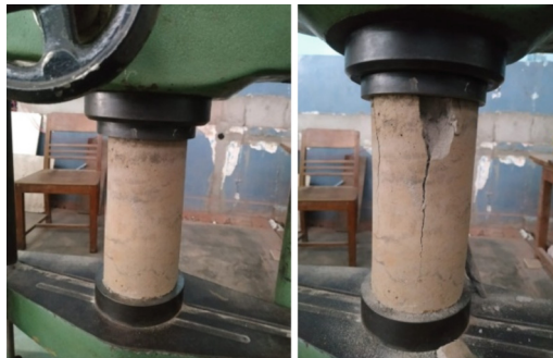
Fig. 9. Bottom ash based backfill under UCS test.
