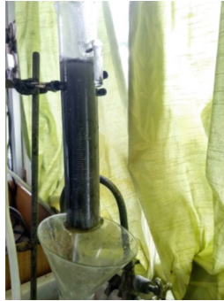
Fig. 11. Constant head permeameter.
