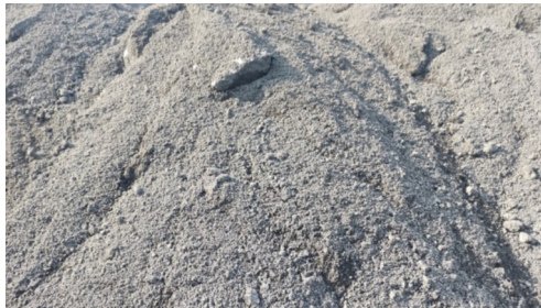
Fig. 12. Granulated slag produced by a charge chrome plant.
