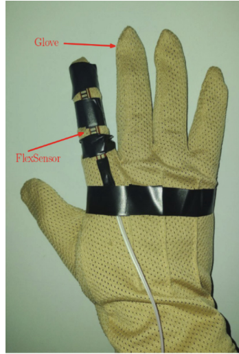
Fig. 2. Glove with embedded FlexSensor for position measurement from the phalanx.
