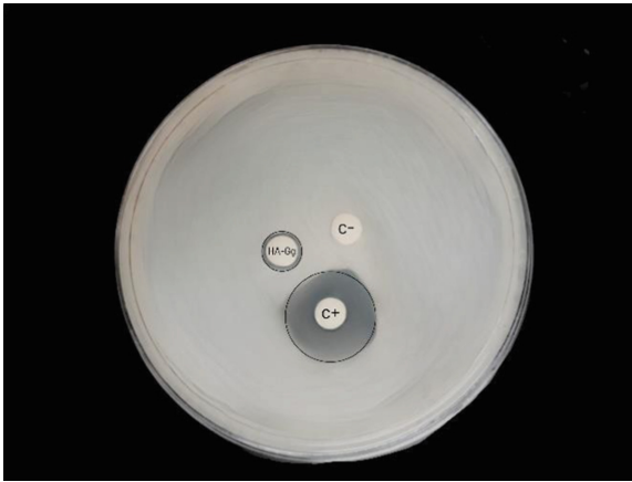
Fig. 4. Result of the antimicrobial activity test by the disk diffusion method using HAp-Gd 0.1 mg/ml against the positive (ciprofloxacin) and negative (water) control.
