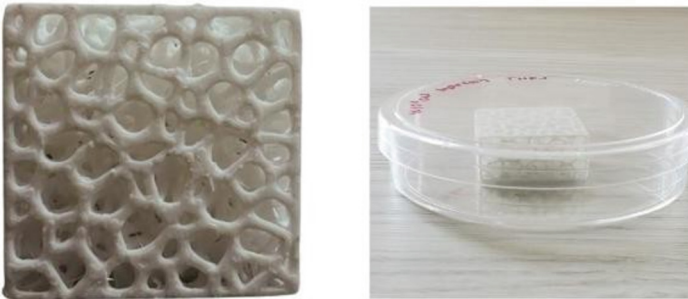
Fig. 5. 3D Scaffold proposal printed at a scale 2:1 for testing probes.
