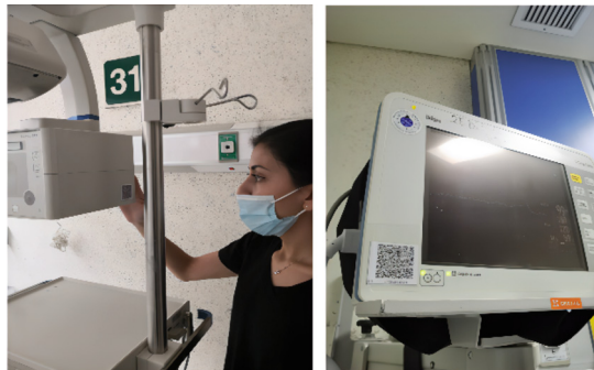
Fig. 4. Deployment of implemented QR codes. Left: The application of QR codes to each piece of medical equipment. Right: The QR code visibly applied on a vital signs monitor, ready for use.
