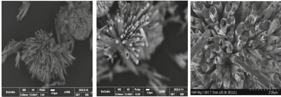
Fig. 2. Microphotographs of magnesium-doped hydroxyapatite obtained by SEM at different magnifications.
