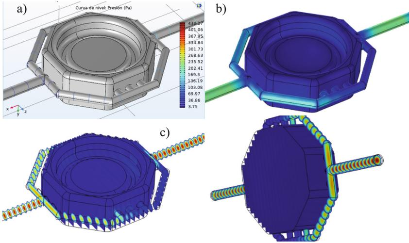
**Fig. 3.** Navier-Stokes COMSOL solver of the microfluidic biological system. Flow simulation components. a) System Volume with conditions. b) Chamber flow fields and their distribution. c) Vectors fields through the support in the form of the chamber.
