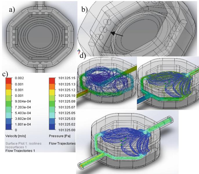
**Fig. 1.** Components of the microfluidic biological system. a) Top view of the system. b) The pipes and holes of the in vitro test system. c) The top view of the pipes of the in vitro test system. d) preliminary Flow simulation with inlet velocity of  $8.3 \times 10^{-5}$  m/s, value referred to a peristaltic pump; and outlet condition at 1 atm.
