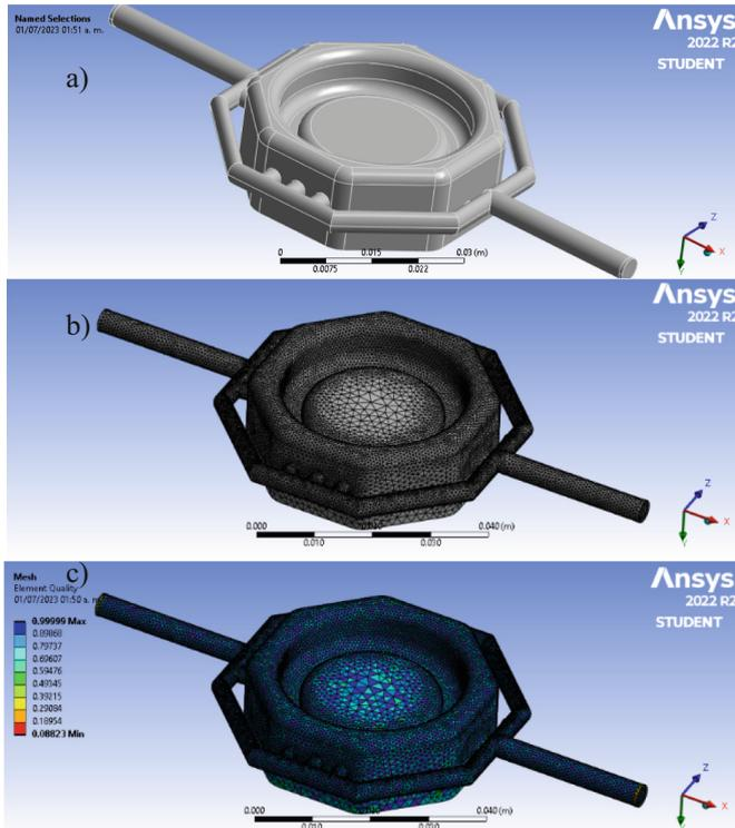
**Fig. 2.** Components of the microfluidic biological system meshed, Fluid volume:  $1.009169 \times 10^{-08} \text{ m}^3$ , Solid volume:  $2.716106 \times 10^{-06} \text{ m}^3$ . a) Volume of the system. b) Generic mesh. c) Element quality and functional cells.
