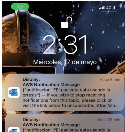
Fig. 8. Screenshot from the cellphone main screen with the email notification telling us that the patient is using the orthoses.
