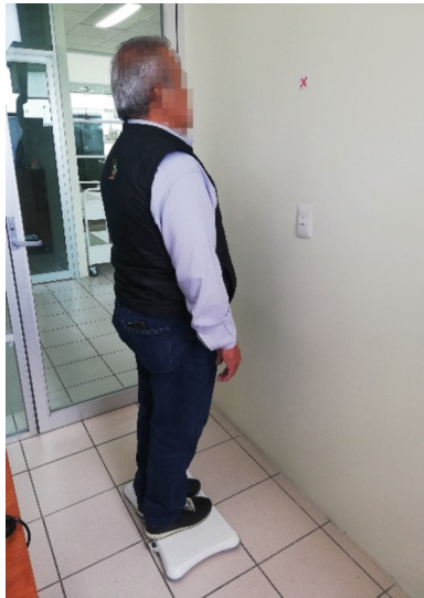
Fig. 6. Subject performing a balance test using the mWBB v1.0 platform
