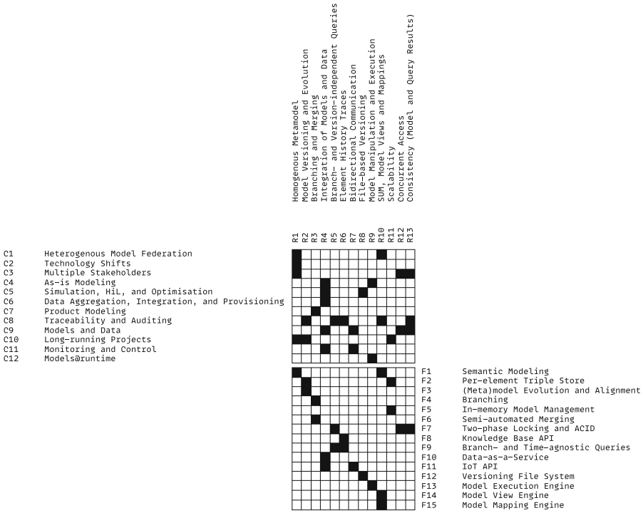
Fig. 2. Traceability matrices between context, requirements, and features.
