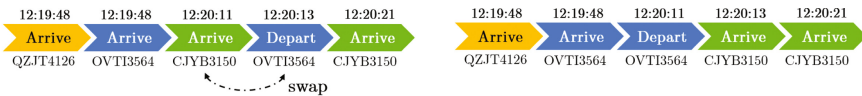
(a) Event data with sensor fault, where a package arrives on the next device before departing the previous device.
