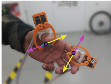
(b) Example of rotational patterns. The purple arrows correspond to the counterclockwise pattern and the yellow arrows correspond to the clockwise pattern.
