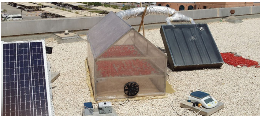
Fig. 29 Experimental setup of a solar PV-powered greenhouse dryer for drying tomatoes (Azam et al. 2020)
