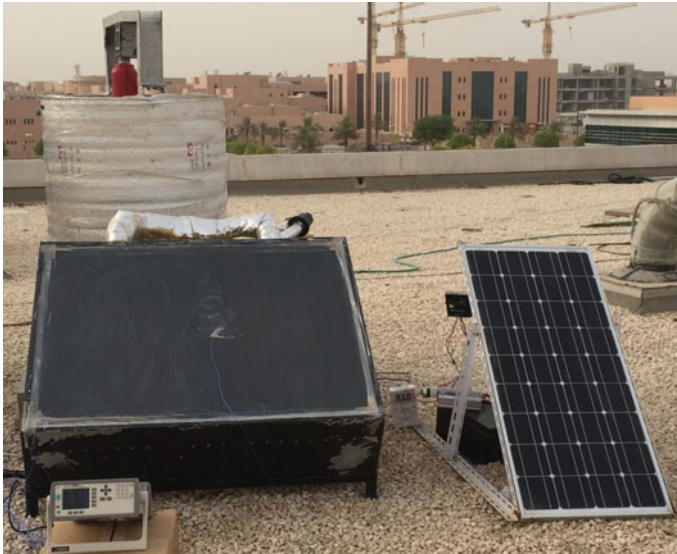
Fig.37 Solar thermoelectric system experimental setup for making date syrup (Air bath with a thermal rocky bed integrated with hydraulic pressure)
