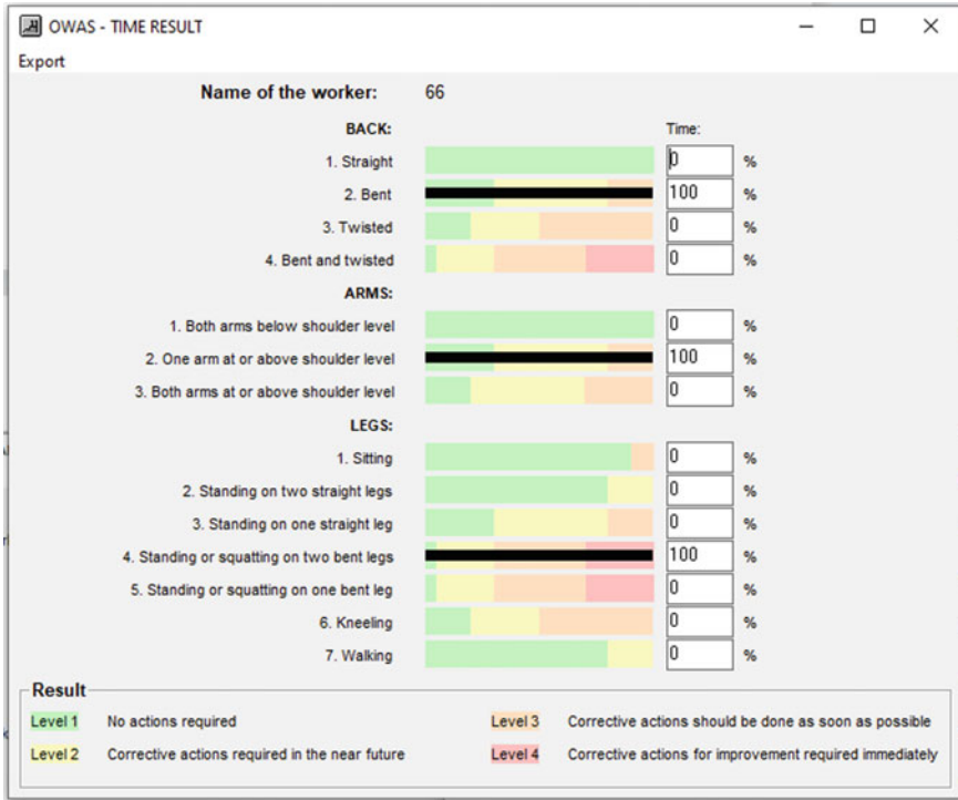
Fig. 7.15 Female worker lifting brass metal (Time result) OUTPUT corrective actions for improvement required immediately
