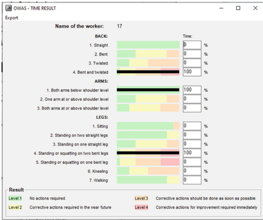
Fig. 7.11 Male worker pouring hot molten metal (Time result) OUTPUT corrective actions for improvement required immediately
