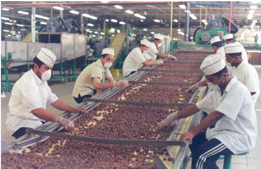
Fig. 4 Dates grading for size and quality inspection prior to bulk packing. Source Dates Processing Factory, Ministry of Agriculture, Alahsa, Saudi Arabia (2002). Source AlKhateeb and Dinar (2002)
