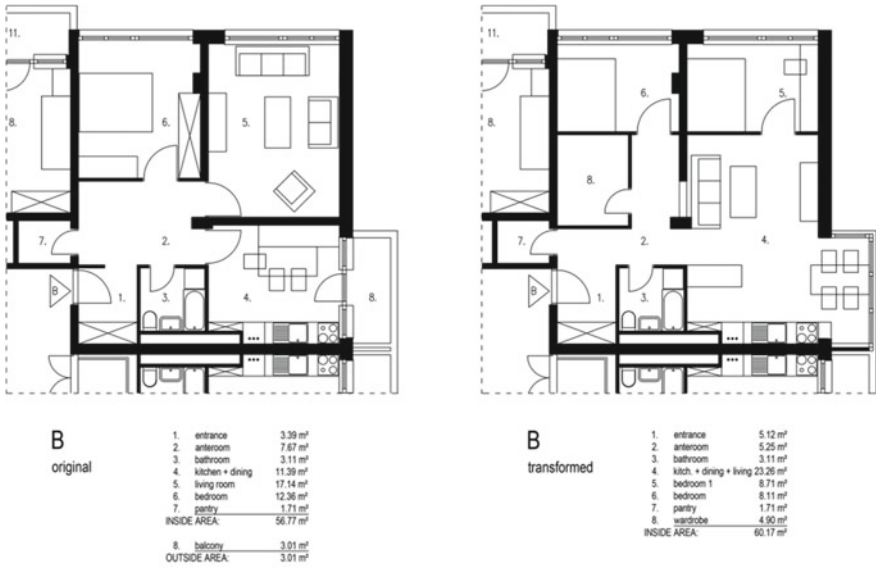
Fig. 7 Original and altered condition found in apartment B with an increased number of bedrooms in the structure of the apartment
