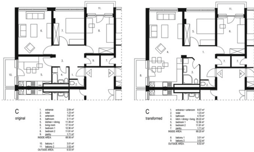
Fig. 8 Original and generally altered condition found in apartment C with combined kitchen, dining room, living room, and extended bathroom
