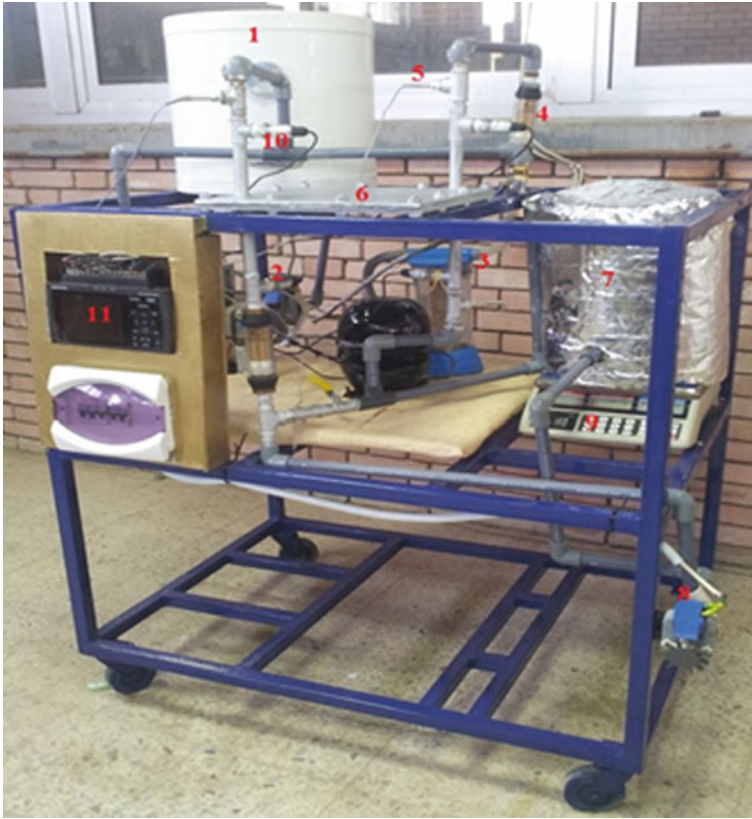
Fig. 2 DCMD experimental unit: (1) heater supply basin, (2) supply pump, (3) filter, (4) rotameter, (5) thermocouple, (6) DCMD unit, (7) permeate tank (with chiller), (8) permeate pump, (9) electronic balance, (10) a pressure transducer, (11) DAQ scheme
