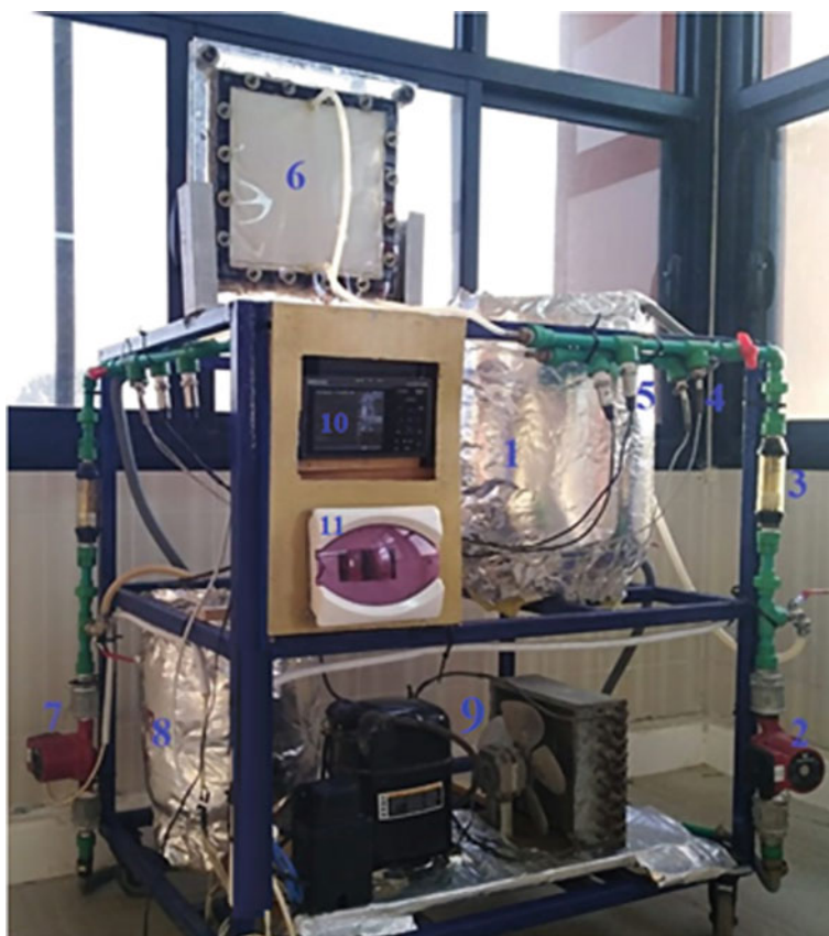
Fig. 2 The actual experimental system utilized in this study; 1—synthetic PW tank, 2—feed pump, 3—rotameter, 4—thermocouples, 5—pressure transmitters, 6—membrane module, 7—cooling water pump, 8—cooling water tank, 9—refrigeration cycle, 10—data logger, 11—electricity panel
