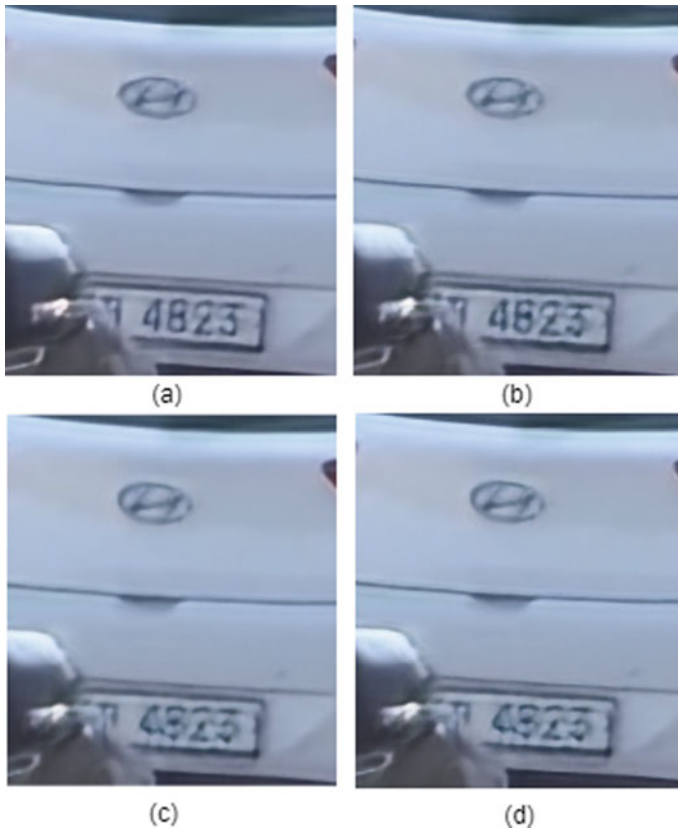
Fig. 3 Results using different patch size; a patch size = 3 \times 3 , b patch size = 5 \times 5 , c patch size = 7 \times 7 , d blurry input image
