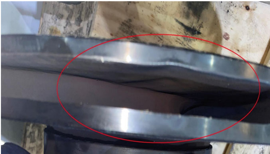
Fig. 9 A bend on the internal blades of the impeller
