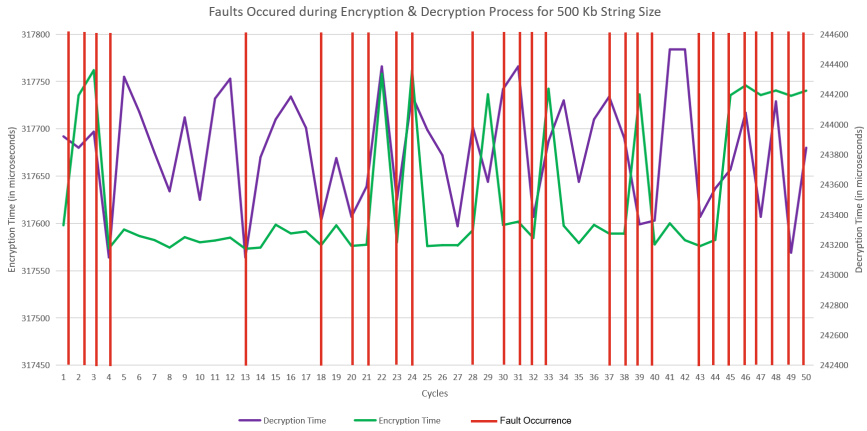
Fig. 8. Fault Occurrence for Encryption & Decryption Processes for a 500 Kb String Value
