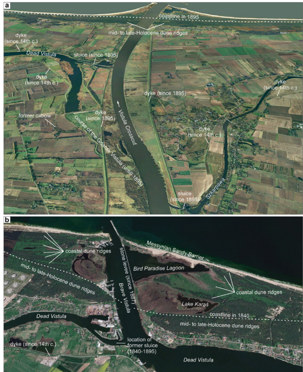
Fig. 42.5 Pseudo-3D geovisualization of selected Vistula River mouths. Source: Google Earth Pro; due to the oblique view not to scale. a The Vistula Crosscut—an artificial mouth made in 1895; the Gdańsk Vistula has been cut by a dyke with sluice and renamed to the Dead Vistula. b Brave Vistula—a natural river mouth formed in 1840, when the Gdańsk Vistula was ice-jammed and the river itself drained a path through mid- to late-Holocene dune ridges of the Vistula Sandy Barrier. It remained active until the opening of the Vistula Crosscut
