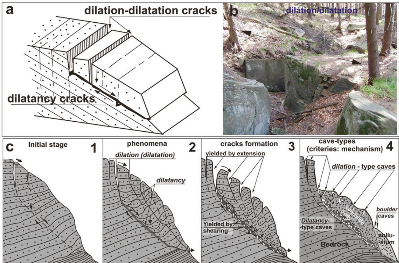
**Fig. 19.2** The conceptual model of formation of non-karst caves due to dilation (dilatation) and dilatancy phenomena. **a** Cracks formed owing to dilation and dilatancy phenomena in hypothetical slope. **b** Trenches formed in effect of dilation (sandstones of the Magura Beds, Mt. Wierch nad Kamieniem, Beskid Sądecki Mts.). **c** Stages
