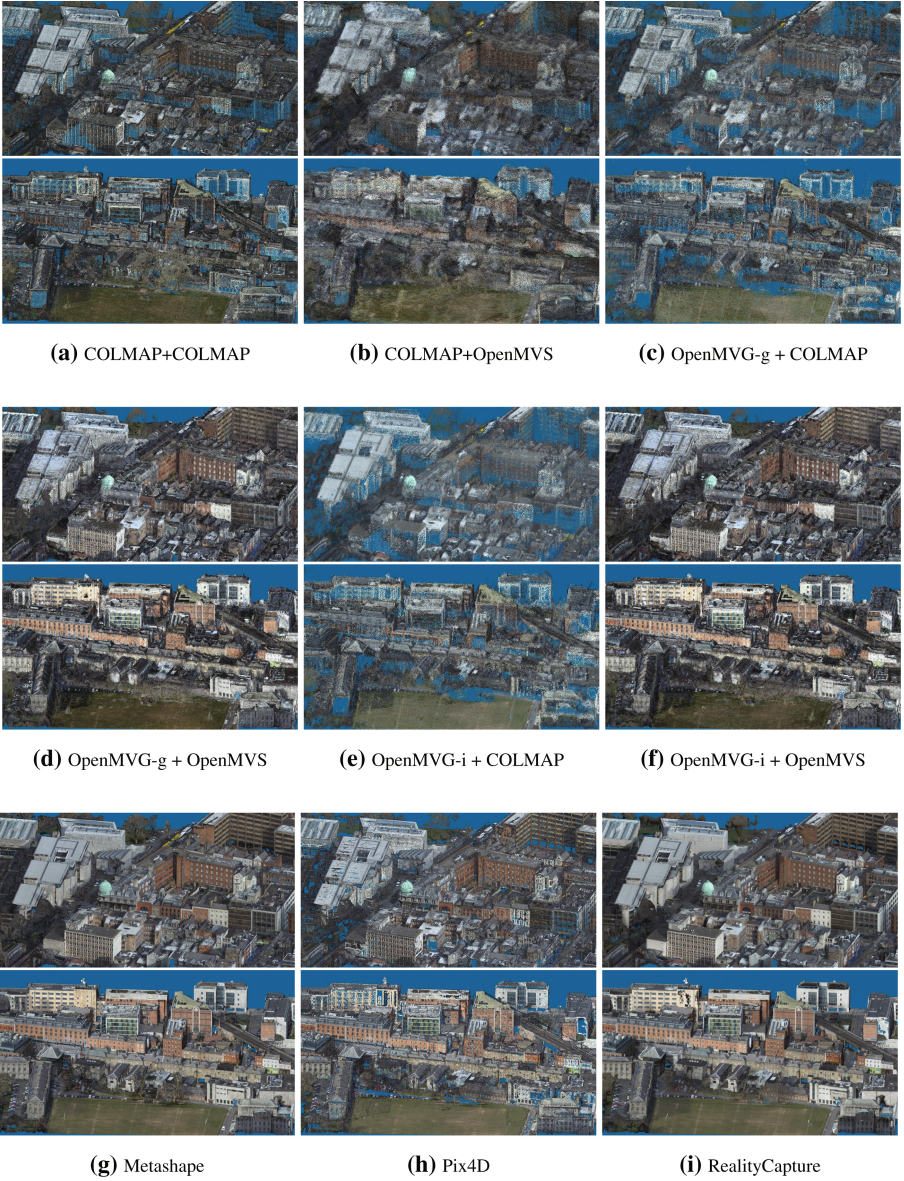
Fig. 5. Qualitative 3D reconstruction results. Point clouds obtained with the oblique and nadir images combined in Area 1 (top) and Area 2 (bottom).
