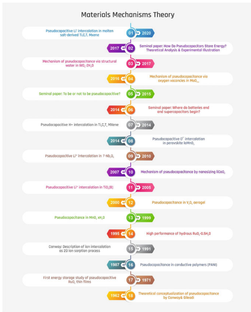
Fig. 2 Pseudocapacitance timeline: novel materials, processes, and theoretical notions
