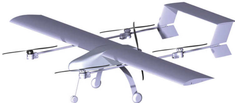
Fig. 9.9 Tardis VTOL UAV with conventional fixed tricycle landing gear
