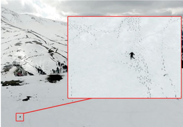
Fig. 5.2 When any image that was judged to be representative of the mannequin was detected, the drone began descending to sharpen the image (Karaca et al. 2017)
