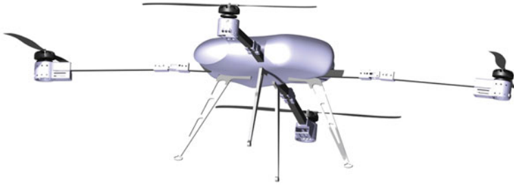
Fig. 9.8 Smartquad UAV with pods from fuselage landing gear configuration
