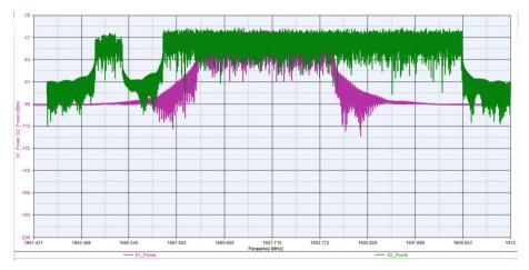
Fig. 5. Test of the spectrum during the coexistence of 4G LTE and 5G NR. ( $f_1 = 1.901$  GHz,  $f_2 = 1.902$  GHz)
