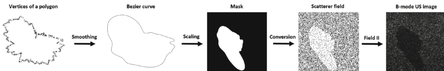
Fig. 1. Ultrasound image generation pipeline. First, a binary mask is generated based on a contour object obtained with a mathematical formula. Next, the binary mask is converted to a scatterer field and Field II simulation tool is used to generate a synthetic b-mode US image.
