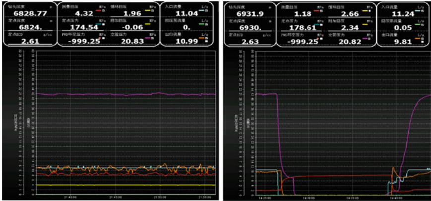
Fig. 9 Wellhead backpressure and flow rate monitor while reaming
