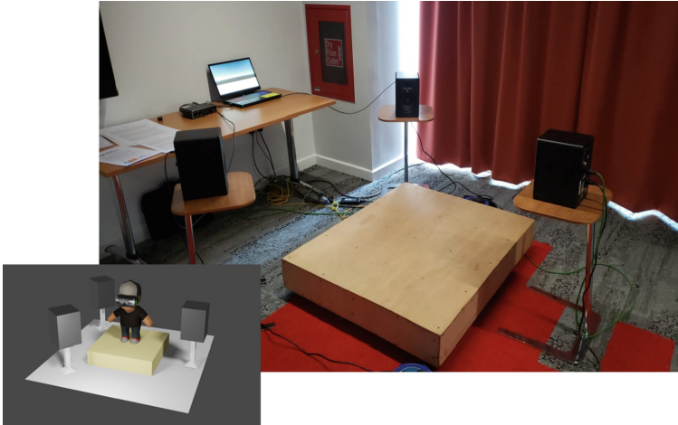
Fig. 1. Proposal for a rig of a sound-based shooting game.
