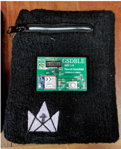
(a) Sweatband with sensor board
