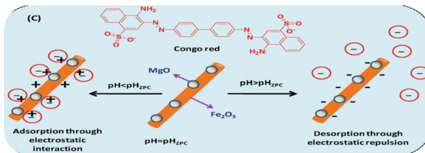
Fig. 2.5 Mechanism of CR extractions on \text{Fe}_2\text{O}_3 -MgO surface by electrostatic interaction [95]. Copyright 2020. Reproduced with permission from Elsevier
