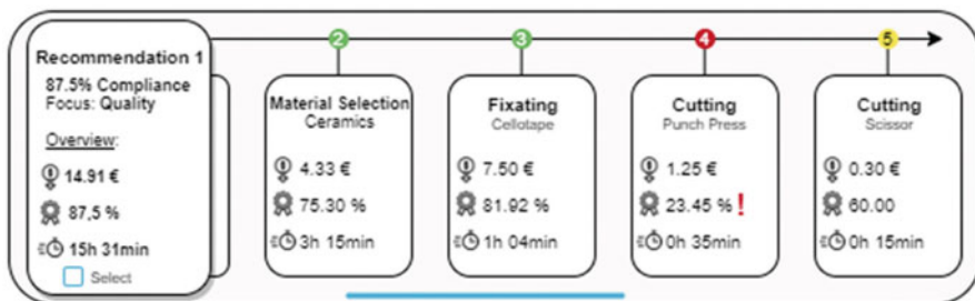
Fig. 5.9 Illustration of a recommended process configuration from the FRP process chain planning tool with a global evaluation of the whole chain on the left and local information on possible problems on the right
