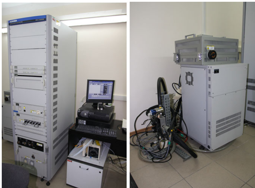
Fig. 11 Gas analysing complex MEXA-7400DEGR
