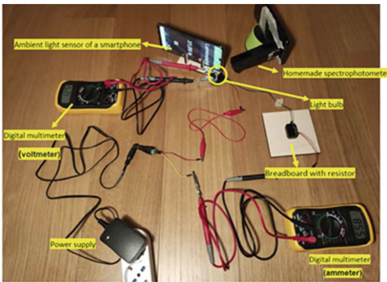
Fig. 2 Experimental apparatus for quantitative experiments about blackbody radiation (Onorato et al. 2021a, b) as photographed by one of the students
