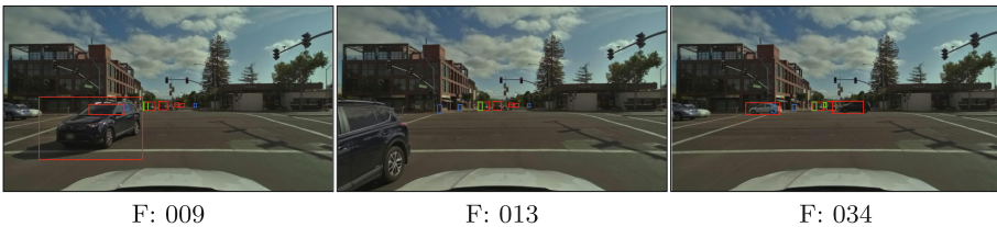
Fig. 5. The results of running Query 2 through STREM on the Woven Planet (“L5”) Perception dataset. From left to right, the matching frames include an instance of a car (red) occluding a pedestrian (blue), a pedestrian , and a car occluding a pedestrian .
