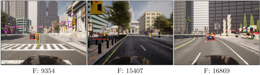
Fig. 6. A series of matching frames with object detections within the CARLA simulator where a pedestrian and vehicle intersect as expressed in Query 3.
