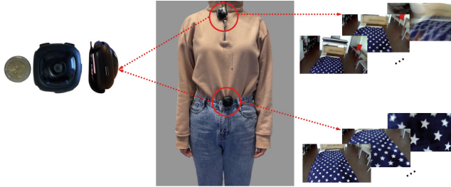
Fig. 1. Mounting of two cameras to the neck and waist of the participant. Left: front and profile photos of the camera compared to the size of a coin. Right: frame sequences collected by the wearable cameras from the two perspectives.
