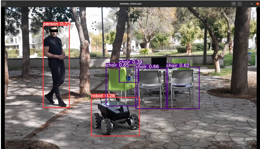
Fig. 6. YOLOv5 detection in an outdoor environment with 25% confidence on robot and 72% on human.
