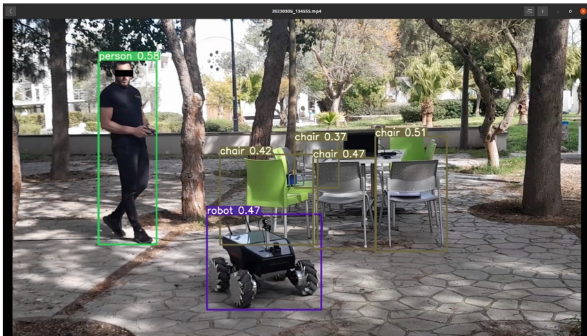
Fig. 7. YOLOv7 detection in an outdoor environment with 47% confidence on robot and 58% on human.
