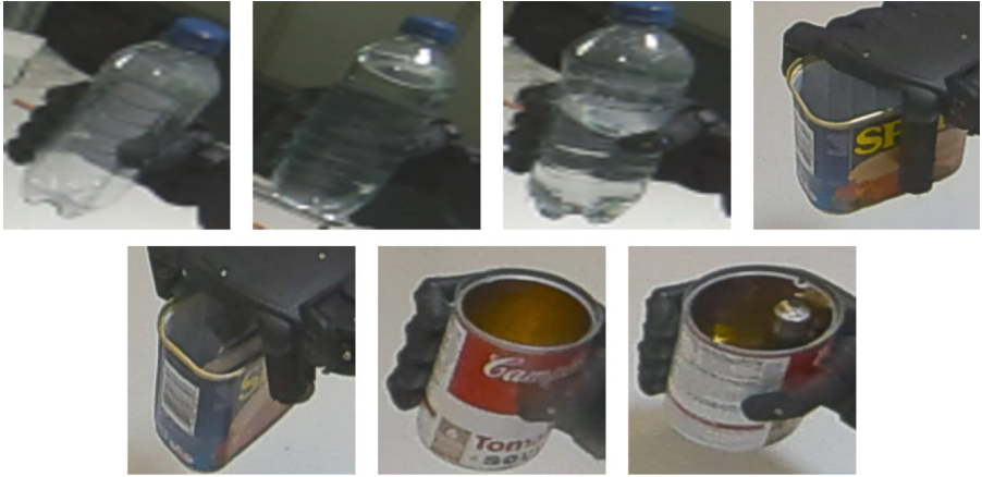
Fig. 1. The seven object classes, from left to right, we have: the empty bottle, the filled bottle, the half filled bottle, the empty spam box, the filled spam box, the empty tomato can and the filled tomato can.
