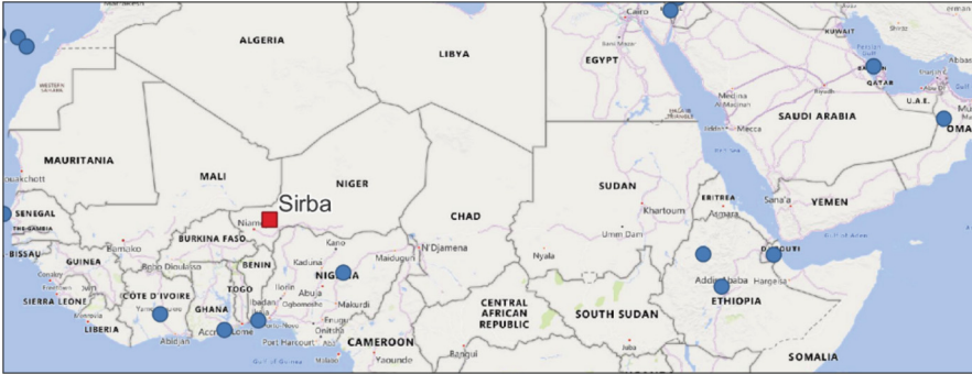
Fig. 1. CORS in north Africa. The blue dots indicate the stations that provide observations to the International GNSS Service (IGS), while the red square is the study area. Data Source: International GNSS Service (IGS), ( https://www.igs.org/ ). (Color figure online)
