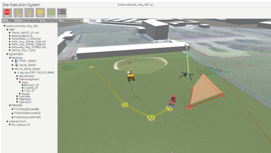
Fig. 3. User-Interface for the SES with three construction machines, restricted areas (red) and a target trajectory (yellow). (Color figure online)
