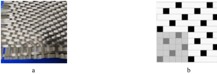
Fig. 19.28: A sample of the CF fabric with the 5/2 satin weave for manufacturing the prepreg (a); a laying pattern for the prepreg (b).
