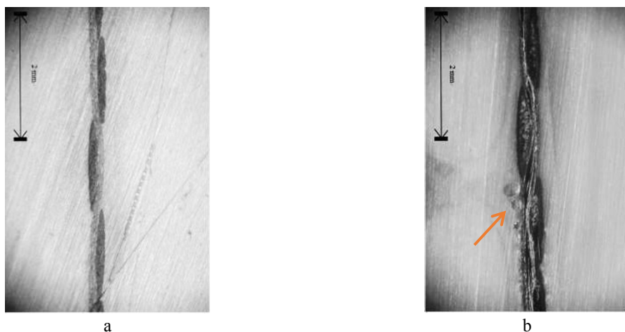
Fig. 19.6: The images of the cross sections of the USW joints with the prepreg thickness of 280 \mu\text{m} ; the USW durations of 800 (a) and 1400 (b) ms.
