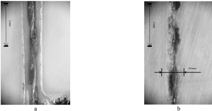
Fig. 19.7: The images of the cross sections of the USW joints with the prepreg thickness of 460\ \mu\text{m} ; the USW durations of 800\ \text{(a)} and 1400\ \text{(b)} ms.
