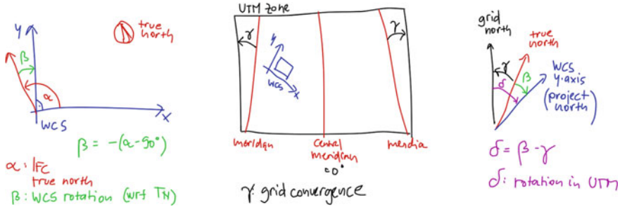
Fig. 4 Calculating rotation from true north when converting via projected CRS
