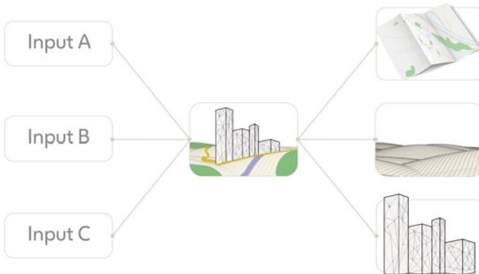
Fig. 2 Representation of the concept for modelling a Digital geoTwin and deriving other geodatasets from it
