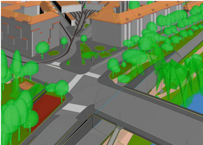
Fig. 20 Detail view of the heterogeneous objects in the test area, modelled using the Digital geoTwin data model developed for Vienna
