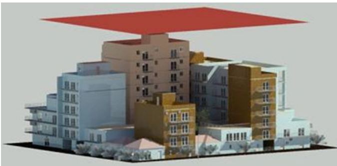
Fig. 9 Construction and height restrictions visualization as 3D surfaces by the experts
