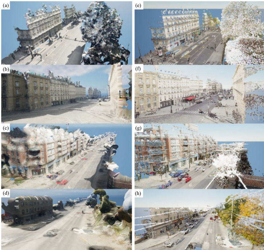
Fig. 4 Mesh visualization of Paris 3D (a, b) and Toronto 3D (c, d). Point visualization of Paris 3D (e, f) and Toronto 3D (g, h)
