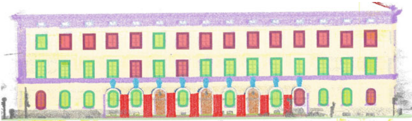
Fig. 13 Correctly (green) and falsely (red) matched windows Reference Data
