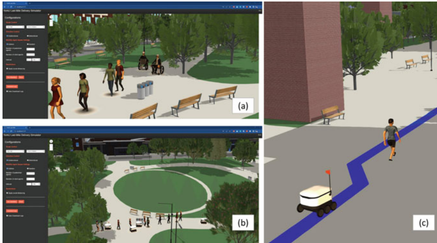
Fig. 8 Last mile delivery robot simulation tool: (a) and (b) show diverse mobility agents, including robots, pedestrians, and wheelchair users, seamlessly progressing to their destinations. In (c), agents adhere to the path created by the route analysis API
