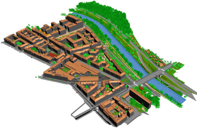
Fig. 21 Overview of the heterogeneous objects in the test area, modelled using the Digital geoTwin data model developed for Vienna
