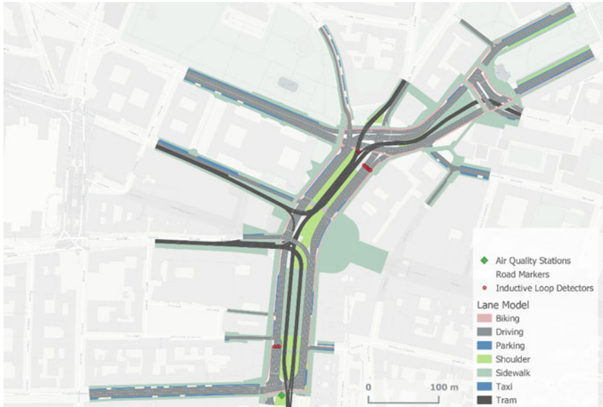
Fig. 2 A map of Boulevard Sonnestrasse showing the street space model, inductive loop detectors and the air quality monitoring station
