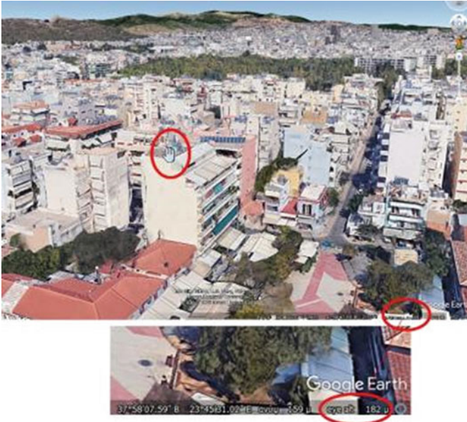
Fig. 1 Approximate elevation measurement (159 m) on the ground surface, in Google Earth Pro Desktop Application
