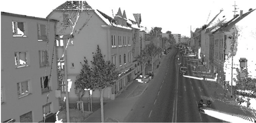
Fig. 3 Example of a 3D cloud captured with a mobile mapping vehicle. The gray-scale values represent reflected intensity
