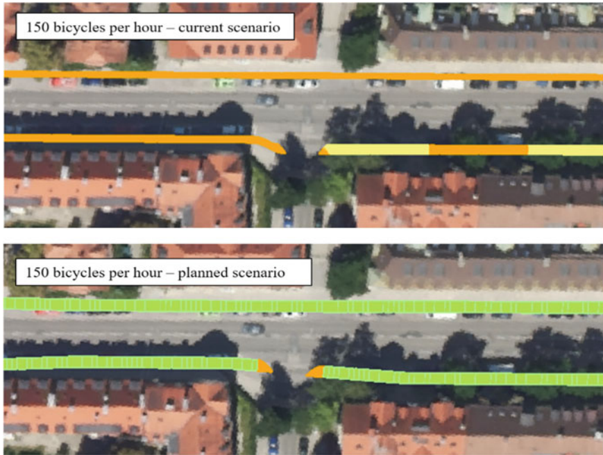
Fig. 5 Comparison of BLOS values at 150 bicycles per hour of the current state of bicycle paths with a planned scenario
