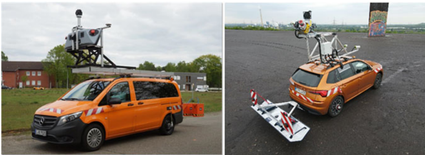
Fig. 1 Two mobile mapping vehicles of the city of Essen with image, video, LiDAR, and ground penetrating radar sensors. The left image shows a Trimble MX8 with GSSI ground penetrating radar horn antennas and the right image an MX9 with a Kontür radar array system
