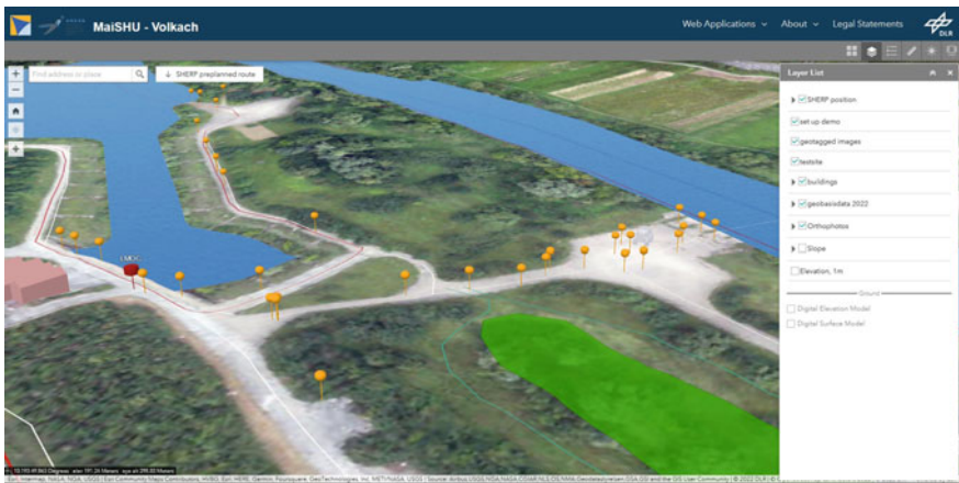
Fig. 5 Screenshot of the demo application. The terrain consists of a digital surface model with a draped orthophoto derived from aerial images together with LoD2 buildings
