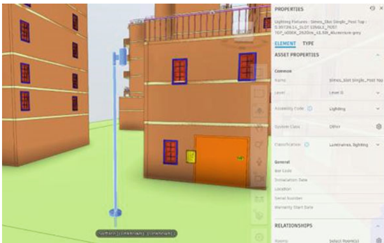
Fig. 25 Classification and functionality of a lighting pole
