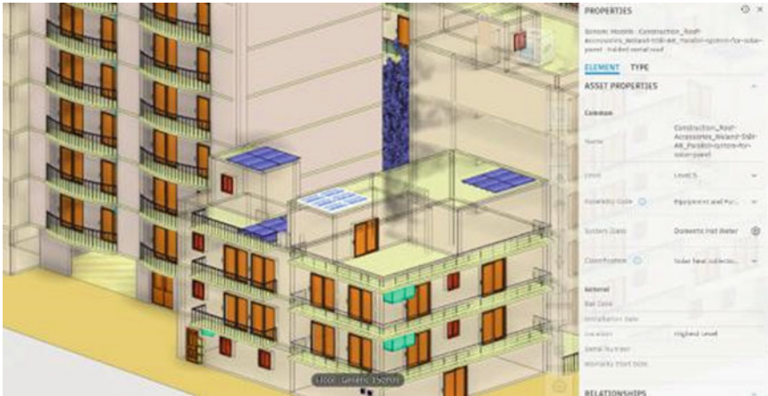
Fig. 26 Semantic categorization of a solar panel unit
