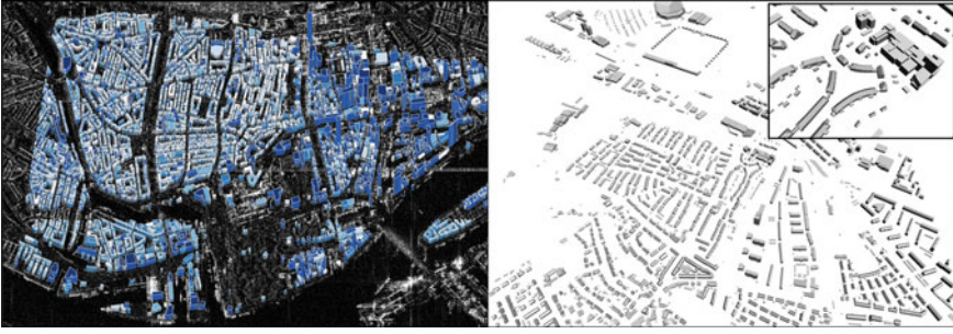
Fig. 2 Multi-scale 3D reconstruction of the built environment. Left: LoD1 building models from TerraSAR-X imagery Sun et al. (2022). Right: LoD2 building models from aerial LiDAR point clouds Chen et al. (2023)
