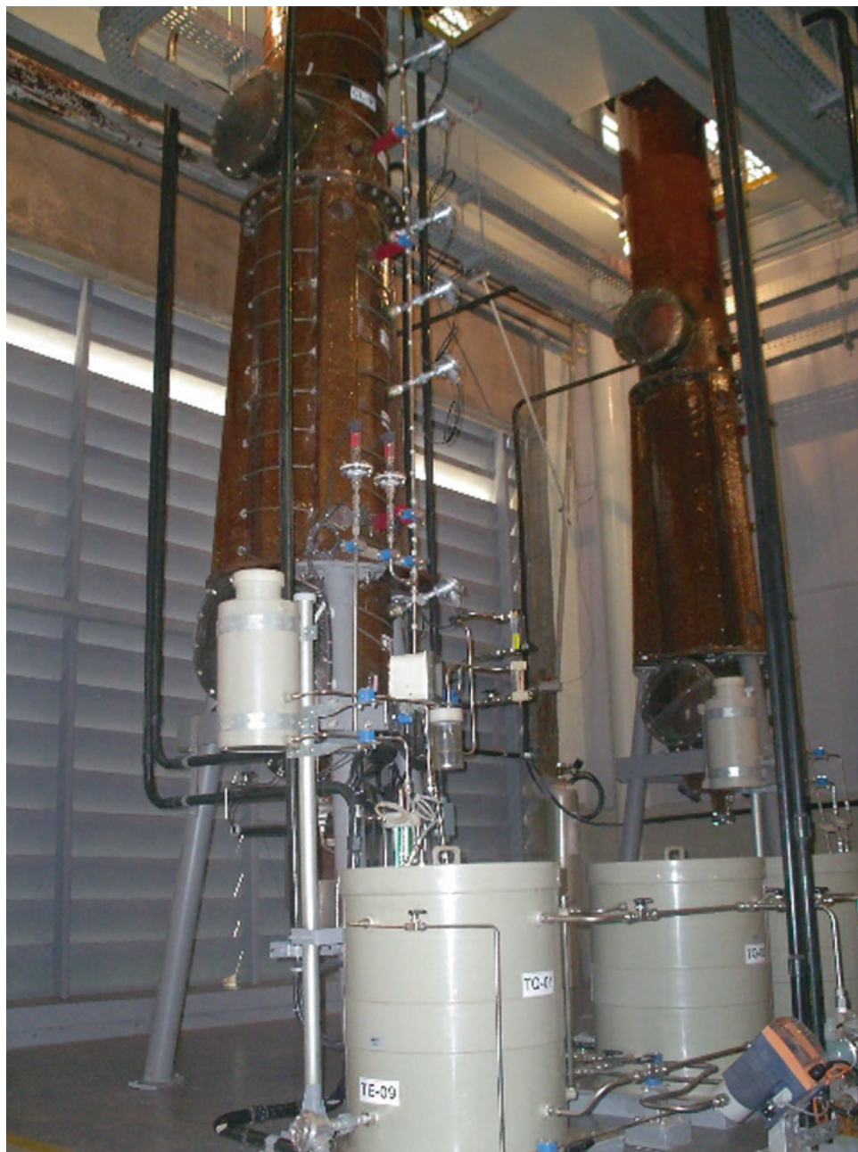
Fig. 14 Pilot plant for the bioleaching of pyrite gravity concentrate designed and assembled at CETEM—Centre for Mineral Technology/Rio de Janeiro/Brazil. Source The authors
