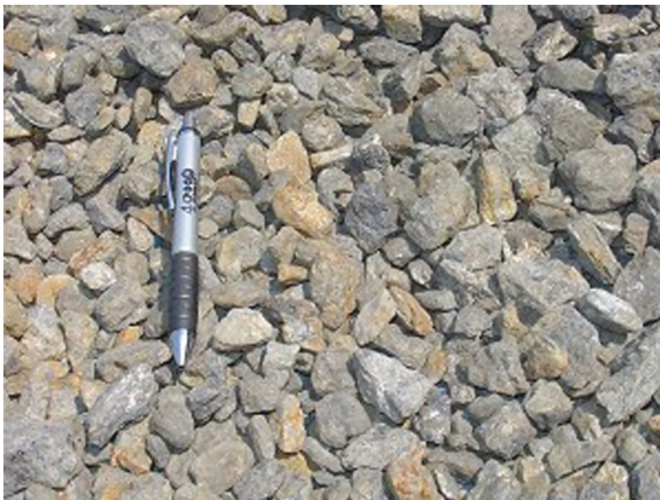
Fig. 13 Sample of pyrite gravity concentrate from a Brazilian coal mine Source The authors
