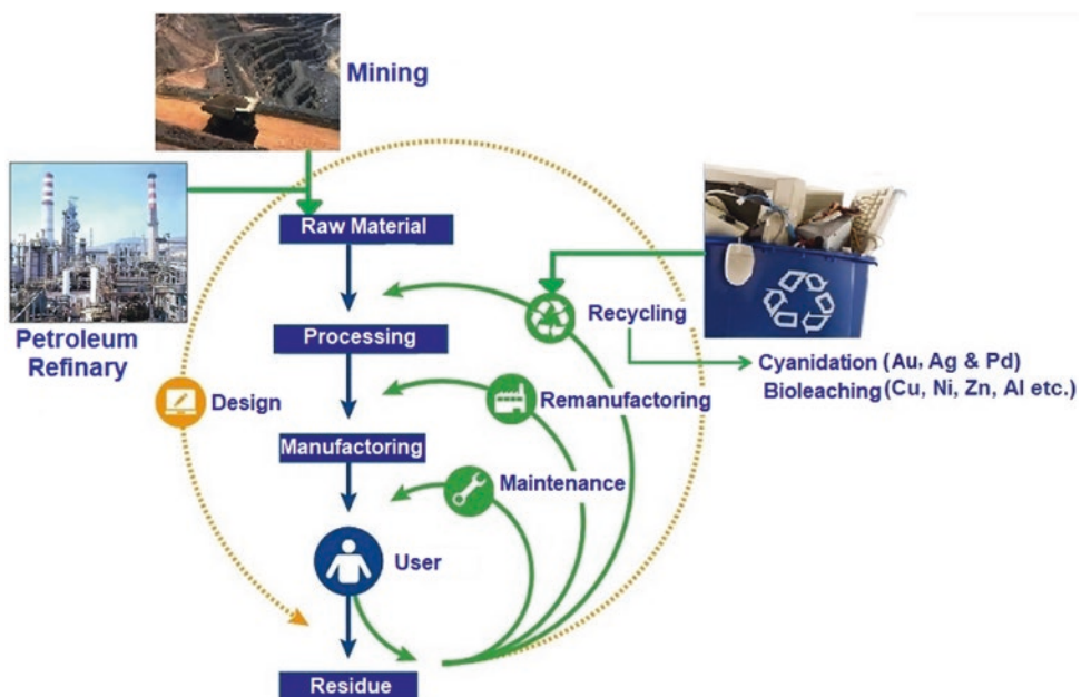
Fig. 7 Production of electro-electronic devices from different natural resources and their post-consume discharge and recycling under the concepts of circular economy. Source The authors
