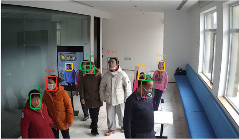
Fig. 7.10 The surveillance scenario. There will be multiple faces involved in the surveillance camera. In addition to regular faces, there will be criminals wearing high-fidelity masks and faces that belong to noise in the background of posters, advertisements, etc
