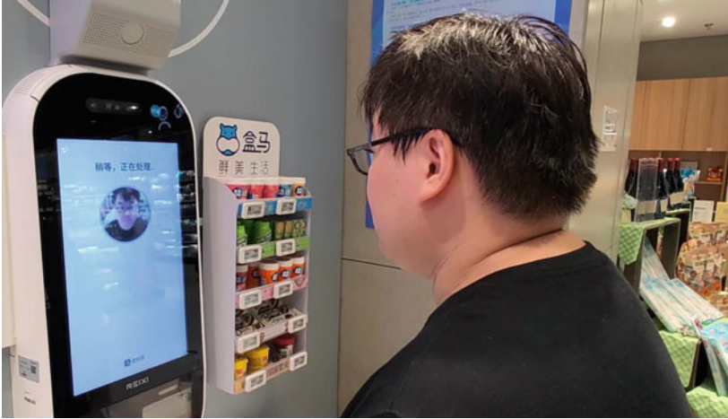
Fig. 7.8 The offline payment scenario. The customer completes a face recognition payment process through an industry-specific machine with a fixed offline location. Such special machines are generally equipped with multi-modalities sensors
