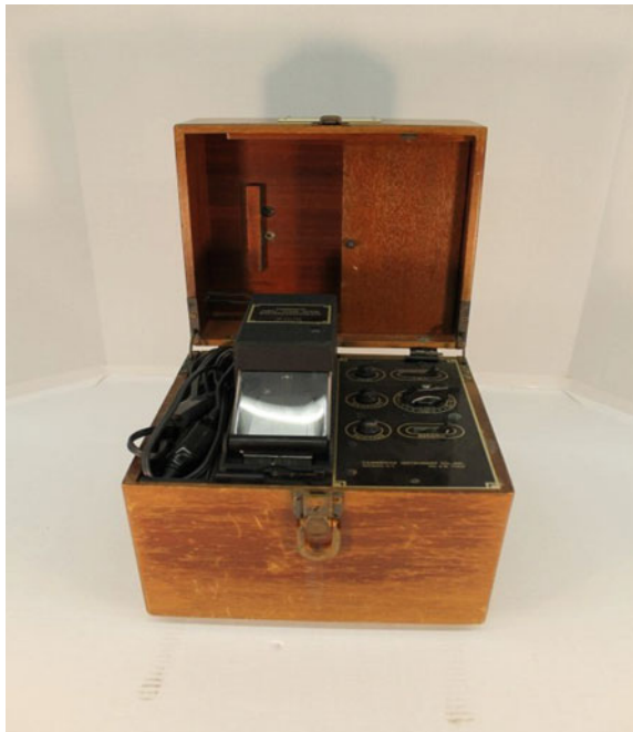
Fig. 2 The Cambridge Simpli Scribe, manufactured from 1945 to 1960. Vacuum tube technology [14]
