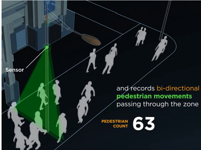
Fig. 3. Diagram of automated pedestrian counting system. Obtained from the City of Melbourne website [19].
