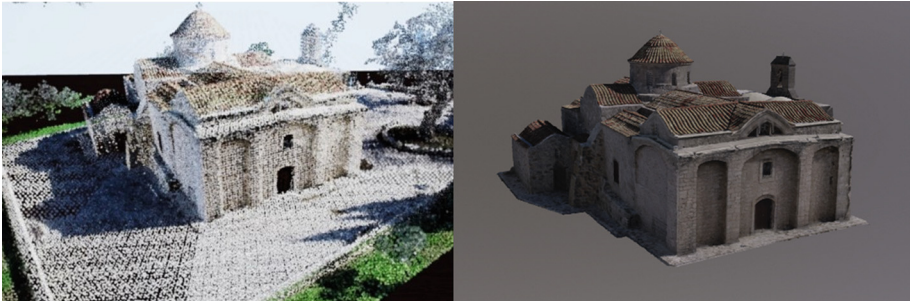
Fig. 1. Point cloud data (left) and 3D generated mesh (right) of the Aggeloktisti church exterior.
