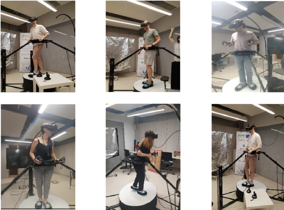
Fig. 7. Human users trying the dynamic fire signage system evacuation routes in the VR environment.
