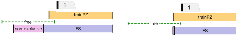
Fig. 7. The reduction of a REGPZ due to a train position report or a free TTD report
