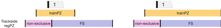
Fig. 6. The extension of a TRAINPZ due to an MA issued within the REGPZ. On the left the TRACKSIDE issues an MA, on the right the train actually receives the MA.
