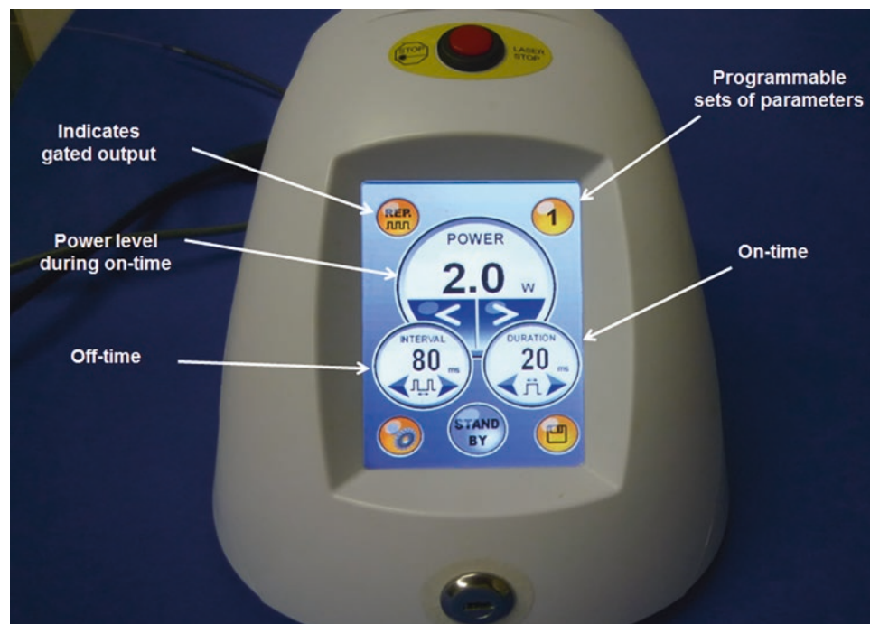
■ Fig. 4.27 This 810 nm diode laser has limited variables that may be controlled directly. It is used here with a 400 \mu\text{m} diameter optical fiber
