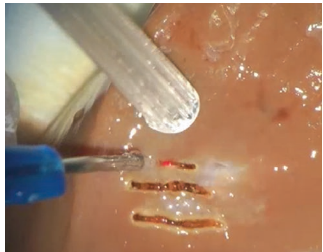
■ Fig. 4.24 Three cuts all performed with a 940 nm diode laser at 1 W, CW. The bottom cut done with no precooling and air or water irrigation. Note the significant collateral damage. The middle cut was performed with air directed over the surface. Speed of cut was slower but as effective with much less collateral damage. Applying an air/water spray during treatment in the top cut caused significant surface cell death. (Courtesy of Dr. Mark Cronshaw)
