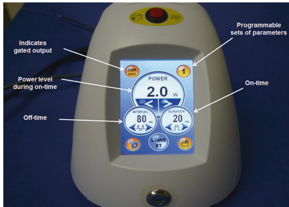
■ Fig. 4.5 This 810 nm diode laser has a limited number of variables that may be controlled directly
