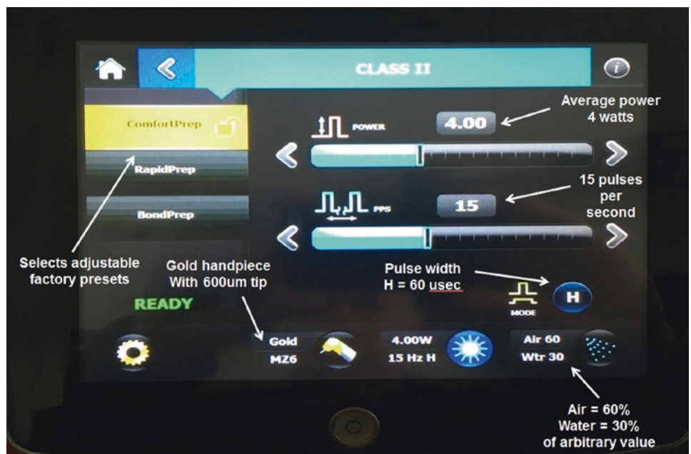
Fig. 4.30 This 2780 nm Er,Cr:YSGG laser has a choice of two pulse widths. It allows control of average power, but energy per pulse and peak power must be calculated. Levels of auxiliary air and water are set as percentage of an arbitrary value
