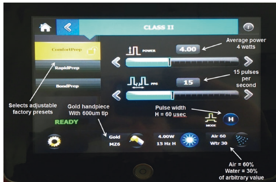
■ Fig. 4.6 This 2780 nm Er,Cr:YSGG laser has a choice of two pulse widths. It allows control of average power, but energy per pulse and peak power must be calculated. Levels of auxiliary air and water are set as percentage of arbitrary values determined by supply to the individual dental suite
