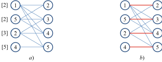
Fig. 2. a) Bipartite graph for 1-union graph in Fig. 1; b) Maximum matching (red bold lines).
